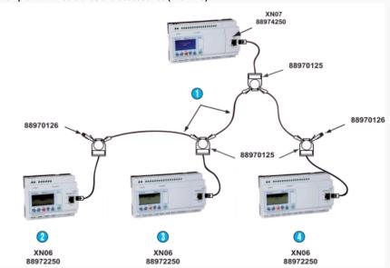
Concerning connection precautions, please refer to the installation sheet IS 0876 (M3 Application note - Modbus extension XN06 and XN07 : Implementation of simplified networks)
