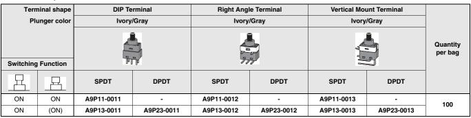
Note: 1. (ON) shows Momentary. ON shows Alternate internally, even plunger is released Momentary.
