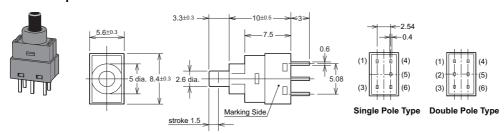
Note: No. (1) and (3) terminals in the SPDT models are dummys to support the Switch case.
