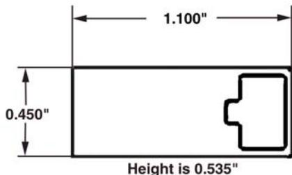
Typical Filtered and Shielded RJ45 Connector
