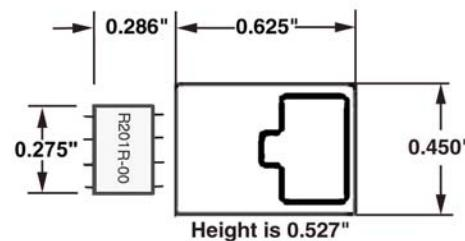
Typical Shielded 4 line RJ45 Connector with
