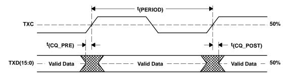
Figure 12. XSBI Transmit Timing Diagram
