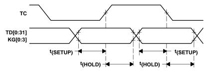
Figure 4. XGMII Transmit Timing
