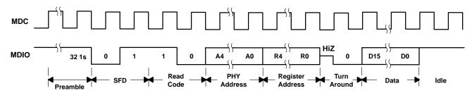
Figure 10. Management Interface Read Timing
