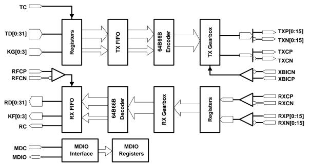
Figure 3. The DLKPC192S Block Diagram
