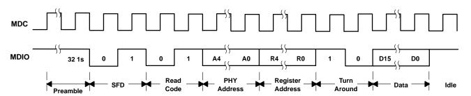
Figure 11. Management Interface Write Timing
