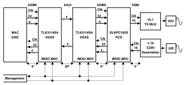
Figure 2. 10-Gbps Ethernet Long-PCB-Distance Implementation
