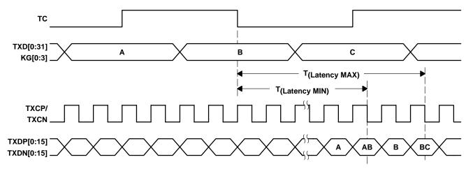
Figure 6. Transmitter Latency
