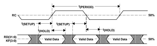
Figure 15. XGMII Receive Timing Diagram
