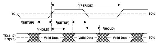
Figure 14. XGMII Transmit Timing Diagram
