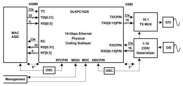
Figure 1. 10-Gbps Ethernet Short-PCB-Distance Implementation
