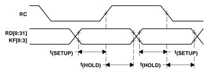
Figure 8. Receive Interface Timing
