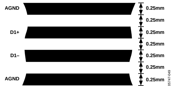
Figure 61. Arrangement of Signal Tracks
