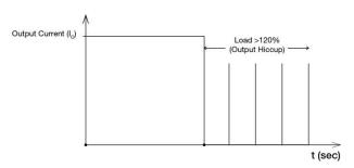
It is not recommended to prolong the duration of  $I_{\rm O}$  when it is <120% but >100%, since it may cause damage to the PSU.
