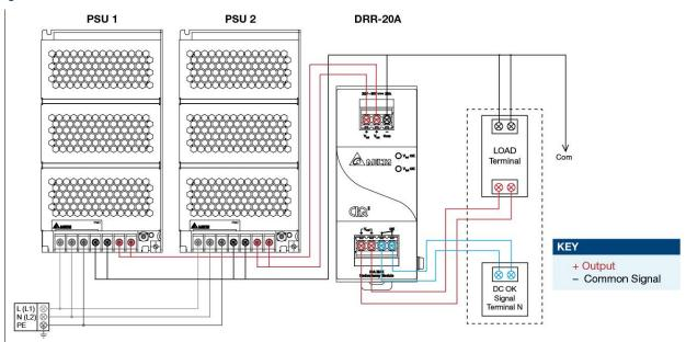
Fig. 3 Redundancy / Parallel Operation Connection Diagram
