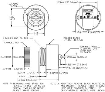
NOTE A: TERMINALS-032 BRASS TIN PLATED, TAPPED FOR #6-32 SCREW. TWD #6-32 NICKEL PLATED BRASS SCREWS INCLUDED, WILL ACCEPT 1/4\* QUICK CONNECT.
