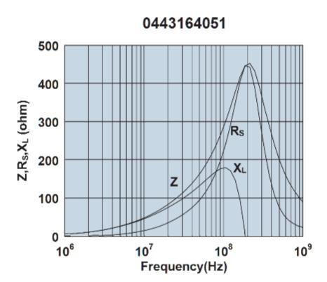
Impedance, reactance, and resistance vs. frequency.
