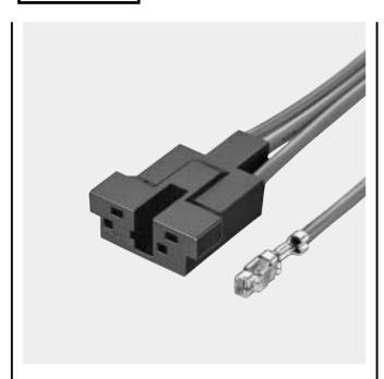
This three circuit connector is used to connect cluster pins {2.3mm (.091") in diameter} to the leads of a motor hermetically sealed in a compressor of a refrigerator or a freezer.
