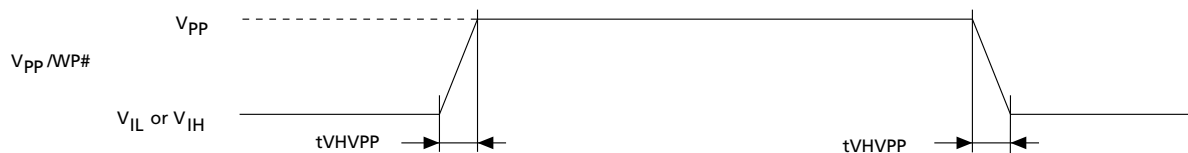
Figure 24: Accelerated Programming Timing Waveform
