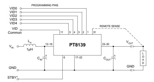
$C_{in}$  = Required 1500 $\mu$ F electrolytic
