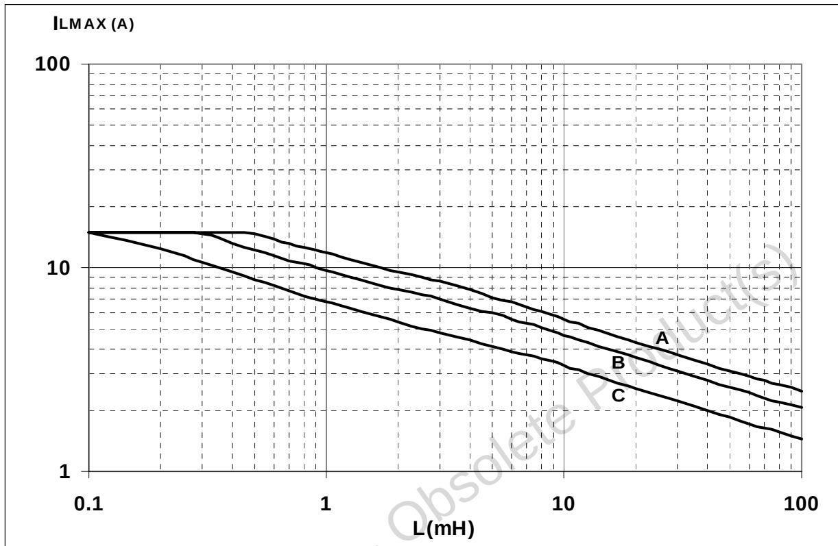
Figure 27. Maximum turn off current versus load inductance
