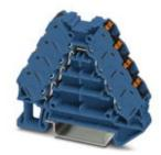
Potential distributors, Nom. voltage: 250 V, Nominal current: 17.5 A, Cross section: 0.14 mm² - 2.5 mm², AWG: 14 - 26, Connection type: Push-in connection, Width: 8.3 mm, Length: 64 mm, Color: blue, Assembly: NS 35/7,5, NS 35/15
