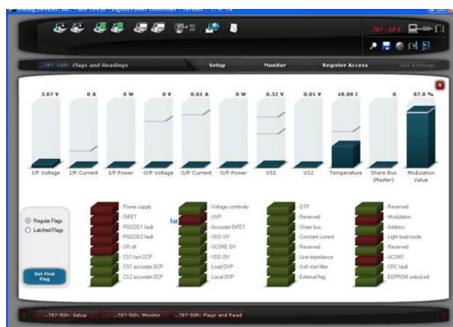
Figure 53 - Corresponding 'Flags and Readings' window. UVP was the first flag that tripped
