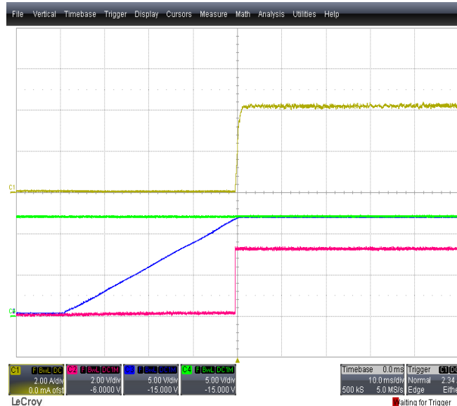
Figure 60 – Output reverse current protection, OrFET enable threshold 0mV Red trace: OrFET gate signal Green and Blue trace: Output voltages of two power supplies Yellow trace: Load current of power supply that is softstarting
