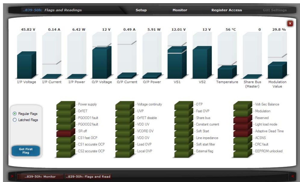
Figure 33 - ACSNS flag tripped during light load mode
