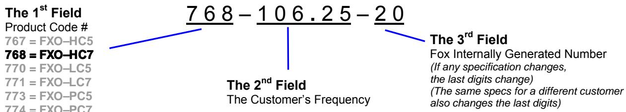
This example, **FXO-HC726R-106.25** = HCMOS Output, Ceramic 7 x 5mm Package, 2.5V, ±25 PPM Stability, -40 to +85°C Temperature Range, at 106.25 MHz
