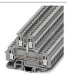
Feed-through terminal block, Connection type: Screw connection, Cross section: 0.2 mm² - 4 mm², AWG: 24 - 12, Nominal current: 24 A, Nominal voltage: 500 V, Length: 62 mm, Width: 5.2 mm, Color: gray, Assembly: NS 35/7,5, NS 35/15, NS 32
