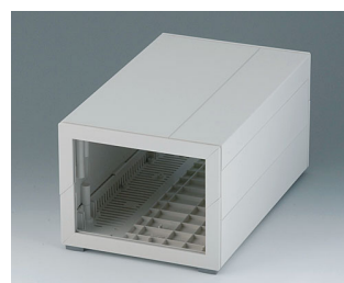
B2212217 MEDITEC E 220, without handle bar ABS (UL 94 HB) off-white RAL 9002 6.30"x10.24"x4.88" IP 40
