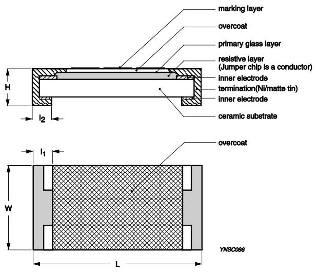
Fig. 4 Chip resistor outlines
