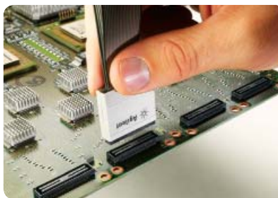
E5385A 34-channel Samtec connector probe
