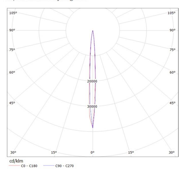
Luminaire: Ledil Oy CP13059\_LOS-RS2 (Osram Square EC 69Im @ 250mA) Efficiency=92% Lamps: 1 x Osram Square EC 69Im @ 250mA
