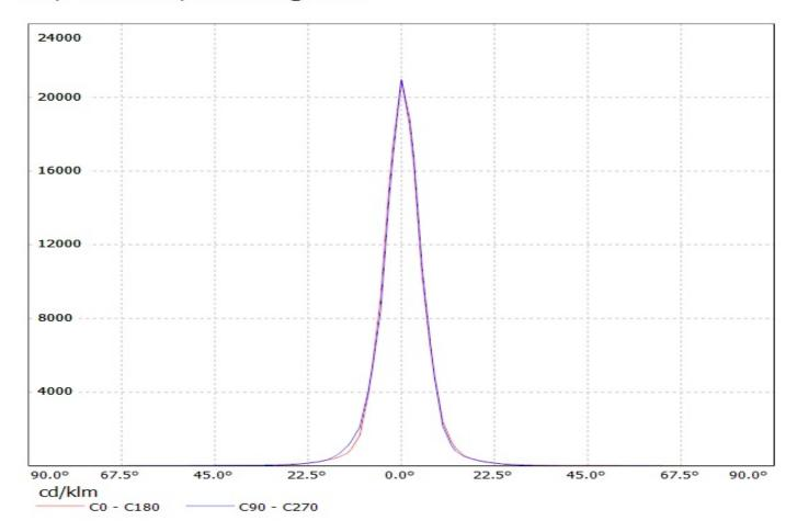
Luminaire: Ledil Oy CP13059\_LOS-RS2 (Osram Oslon 150dg 72lm @ 250mA) Efficiency=93% Lamps: 1 x Osram Oslon 150dg 72lm @ 250mA
