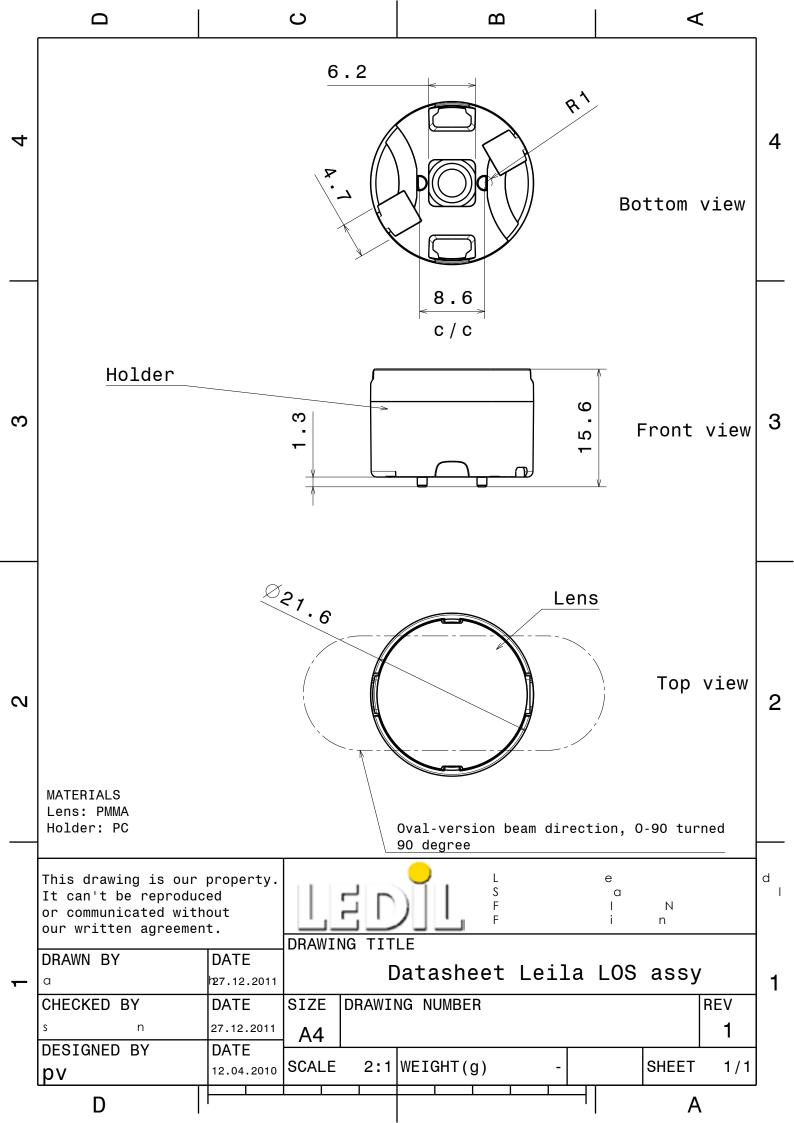
Luminaire: Ledil Oy CP13059\_LOS-RS2 (Osram Oslon 150dg 72lm @ 250mA) Efficiency=93% Lamps: 1 x Osram Oslon 150dg 72lm @ 250mA
