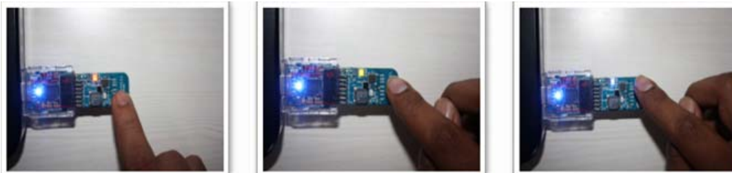
Figure 5-36. LED Color Variation with Respect to Finger Position
