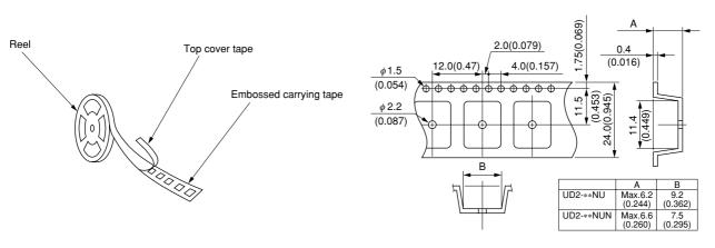
Relay orientation mark and tape carrying direction.
