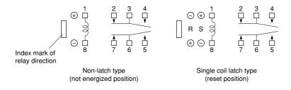
S : Coil polarity of set (operate)
