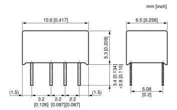
Tolerance of lead pitch is :  $\pm 0.15$  mm [0.006inch] Another tolerance is  $\pm 0.3$  mm [0.012 inch] ( ) is reference value.
