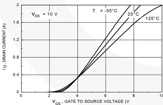
Figure 5. Transfer Characteristics
