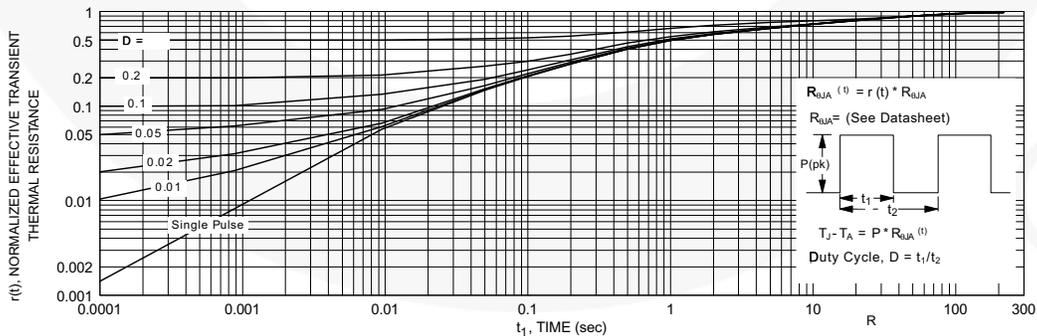
Figure 17. SOT-23, 2N7002 / NDS7002A Transient Thermal Response Curve
