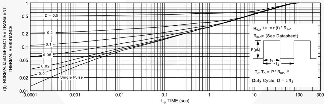
Figure 16. TO-92, 2N7000 Transient Thermal Response Curve
