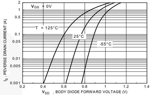
**Figure 8. Body Diode Forward Voltage Variation with Temperature**
