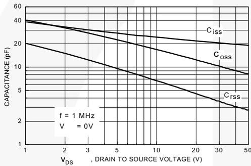
**Figure 9. Capacitance Characteristics**
