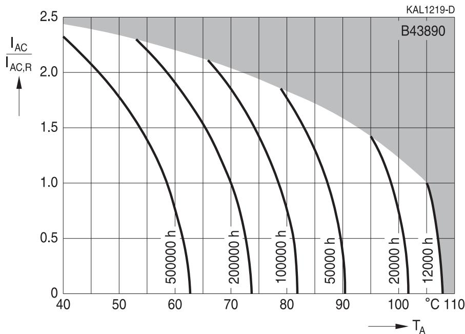
**Useful life<sup>1)</sup>**depending on ambient temperature  $T_A$  under ripple current operating conditions $d \geq 12.5 \text{ mm}$
