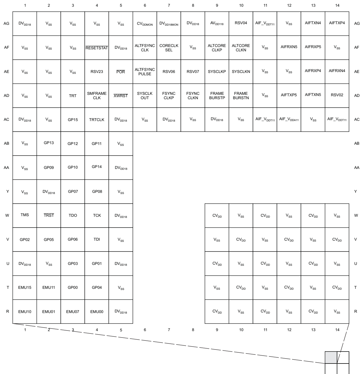
Figure 2-2. C6474 Pin Map (Bottom View) [Quadrant A]
