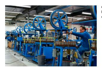
Glenair operates its own high-capacity multispindle overbraiding operation
