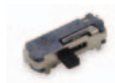
JSM08011SAQNL SPDT Surface Mount Momentary only
