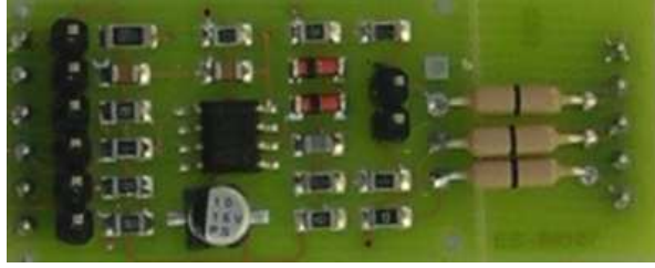
Figure 3.24: The UART RS485 module.
