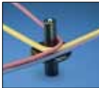
In the "down" position to tie and remove harness.
