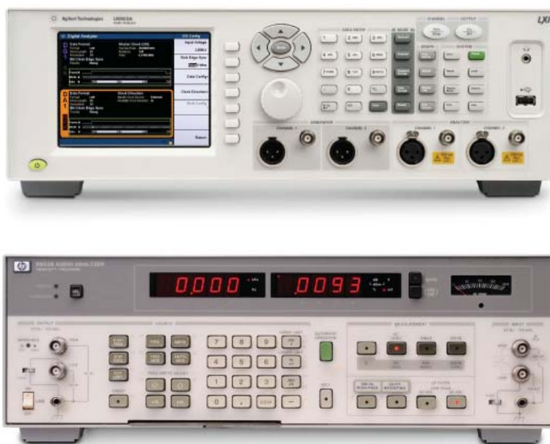
Figure 13. The new U8903A audio analyzer (top) offers numerous improvements over the widely used HP 8903B (bottom).
