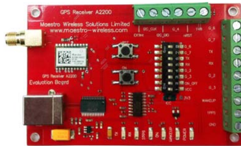
Figure 1: Evaluation board EVA2200-A
