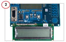
Plug the LCD Module into port P8.
