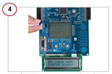
Vary the R56 potentiometer. The voltage is displayed with 16 bits of precision on the LCD module.
