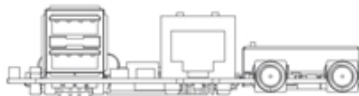
With Ethernet and 2xU.FL connectors, no USB
