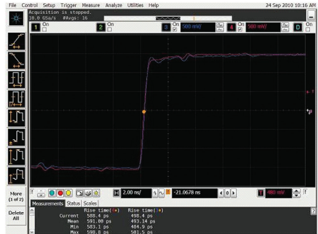
Time domain step response of N2796A (with Agilent MS09404A)
