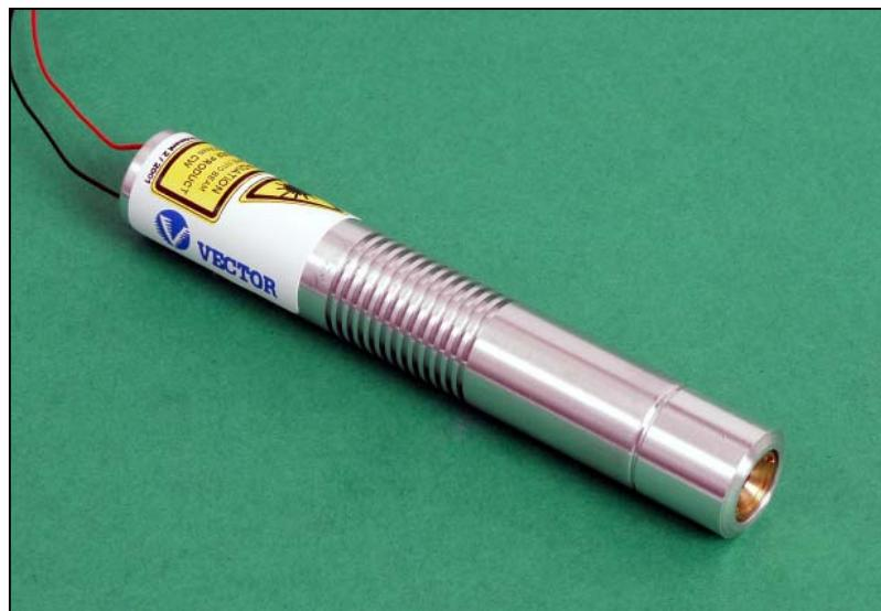
The precision machined housing encloses, protects and stabilises the DPSS laser module, constant current drive circuits and optical assembly. The output beam is shaped by high quality lenses into a narrow, well-defined line or adjustable angle cross.
