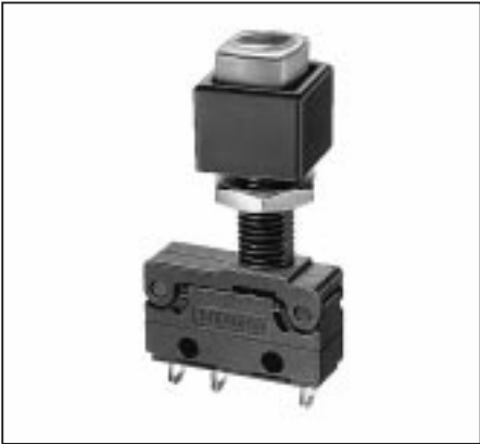
Clip-on frame: Glass fibre reinforced Polyamide (PA 6.6) Bezel: ABS polymer – black Cowl: Synthetic Rubber “O”-Ring: Nitrile Locknut: Brass Nickel plate Button: ABS Polymer Basic switches: V4NC (see pages 36–39) Temperature Range: –10 °C to +85 °C.
