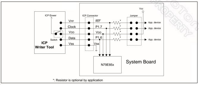
Figure 27-1 ICP Connection with N79E85xA
