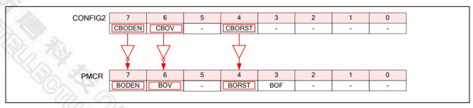
Figure 25–3 CONFIG2 Reset Reloading
