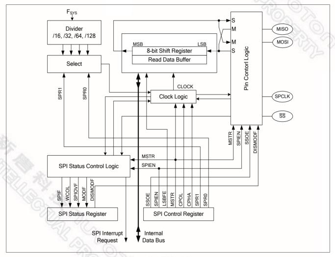
Figure 13-1 SPI Block Diagram
