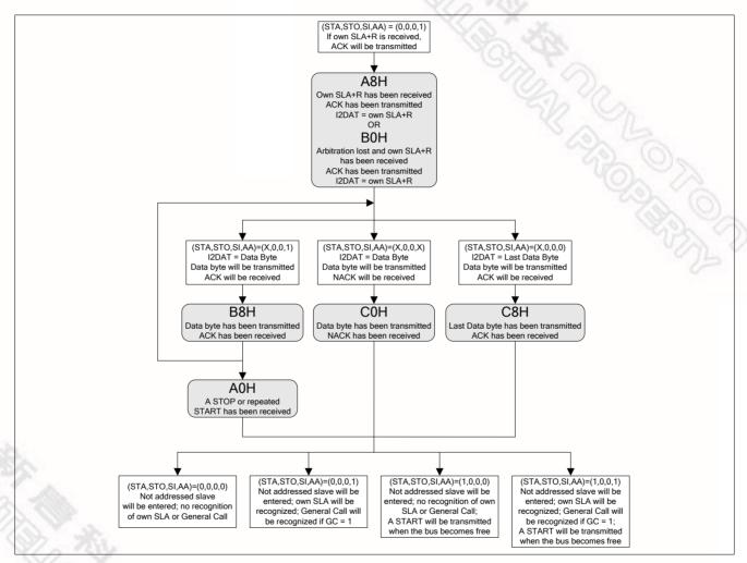
Figure 16-10 Flow and Status of Slave Transmitter Mode
