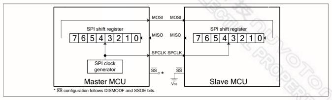
Figure 13-3 SPI Single-master, Single-slave Interconnection
