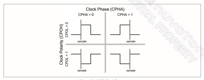
Figure 13-4 SPI Clock Format
