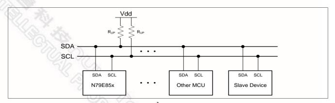
Figure 16–1 I<sup>2</sup>C Bus Interconnection
