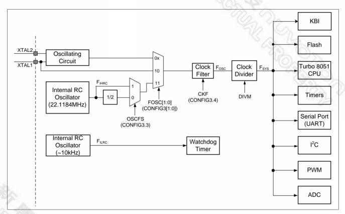
Figure 22-1 Clock System Block Diagram
