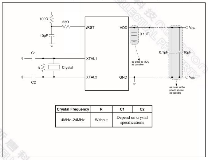
Figure 29-1 Application Circuit for EFT Improvement
