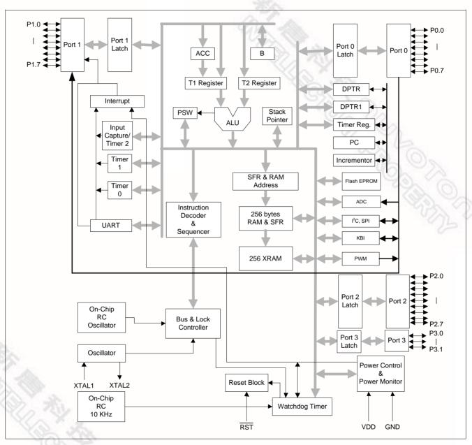
Figure 4–1 N79E855/854 Function Block Diagram
