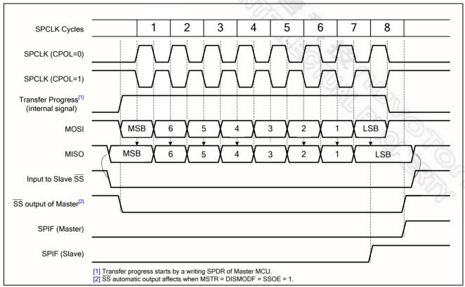
Figure 13-5 SPI Clock and Data Format with CPHA = 0
