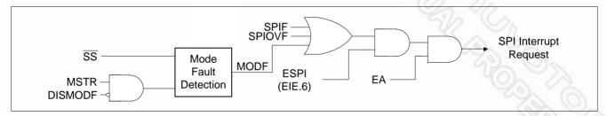
Figure 13-8 SPI Interrupt Request
