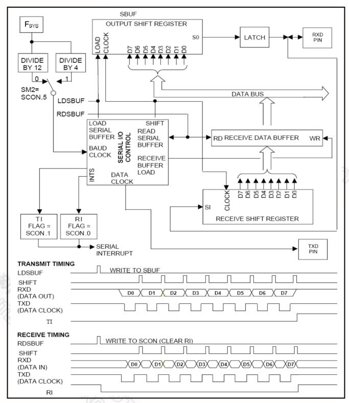
Figure 12-1 Serial Port Mode 0 Function Block
