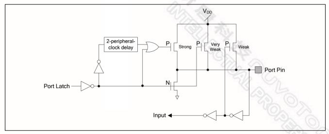
Figure 9-1 Quasi Bi-direction I/O Structure
