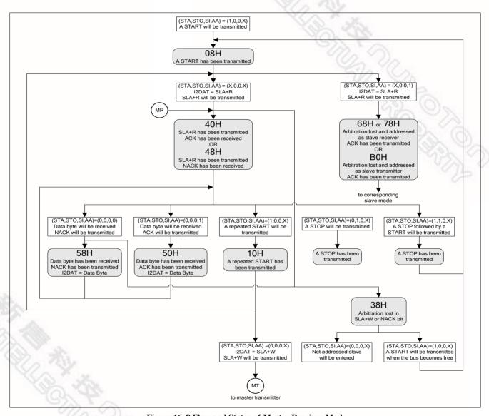
Figure 16–8 Flow and Status of Master Receiver Mode
