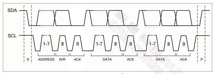
Figure 16–4 Data Format of I<sup>2</sup>C Transfer
