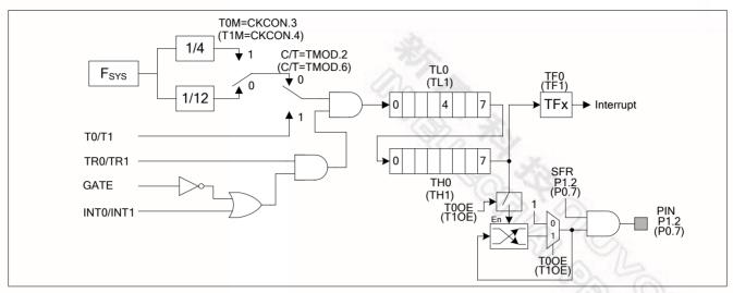
Figure 10-2 Timers/Counters 0 and 1 in Mode 1
