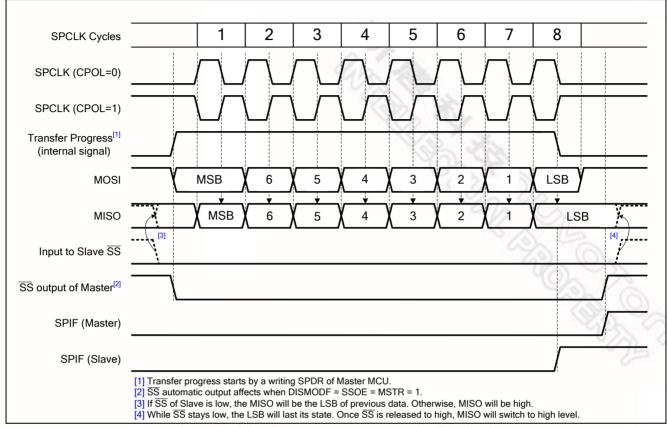
Figure 13-6 SPI Clock and Data Format with CPHA = 1
