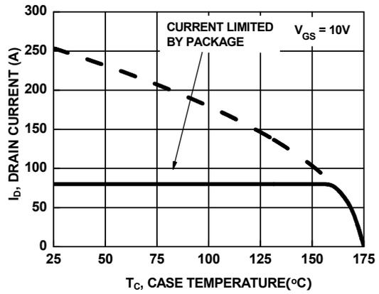
Figure 2. Maximum Continuous Drain Current vs Case Temperature
