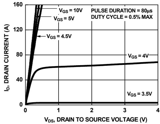
Figure 8. Saturation Characteristics
