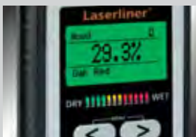
12-position wet/dry LED indicator
