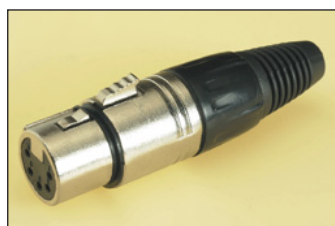
FC6165 5APF/M 5 Pole Female Plug Screw up collet, 6 element cable clamp
