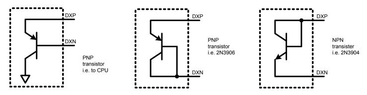
When the thermal sensor is used in a noisy environment, a capacitor can be connected across DXP and DXN to provide some noise filtering capabilities. However, large capacitances affect the accuracy of the temperature measurement. A maximum capacitance of 300pF can be used to help mitigate the noise.
