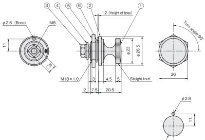
Layout of Hole for Installation
