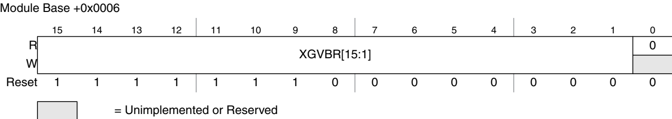
Figure 10-9. XGATE Vector Base Address Register (XGVBR)
