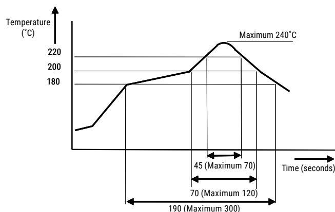
*Note: Temperature profile shows printed circuit board surface temperature on the relay terminal portion.
