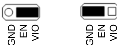
Figure 1. Enable Jumper Settings
