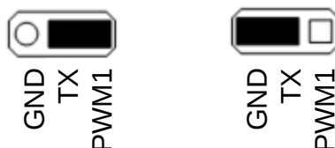
Figure 4. TX Jumper Settings
