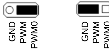
Figure 5. PWM Jumper Settings
