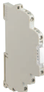
flare 12/24 V DC Input 12/24 V DC Output 1 change-over contact AC 250 V 6 A / DC 300 V 2 A (SPDT)
