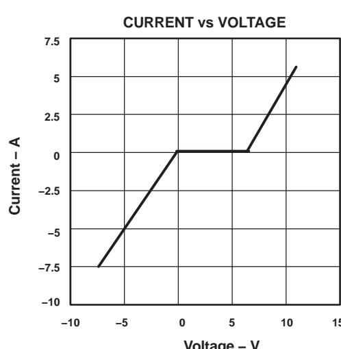
NOTE A: Typical current versus voltage curve was derived using the IEC 1.2/50- $\mu$ s surge waveform.
