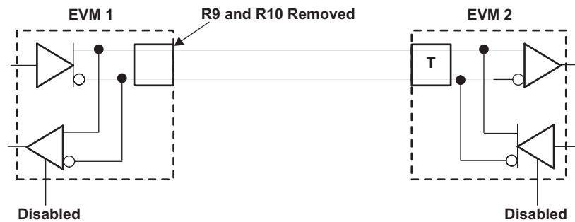
Figure 5. Point-to-Point Simplex Circuit
