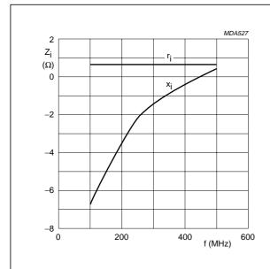
Class-B operation;  $V_{DS}$  = 28 V;  $I_{DQ}$  = 2 × 80 mA;  $P_L$  = 80 W.
