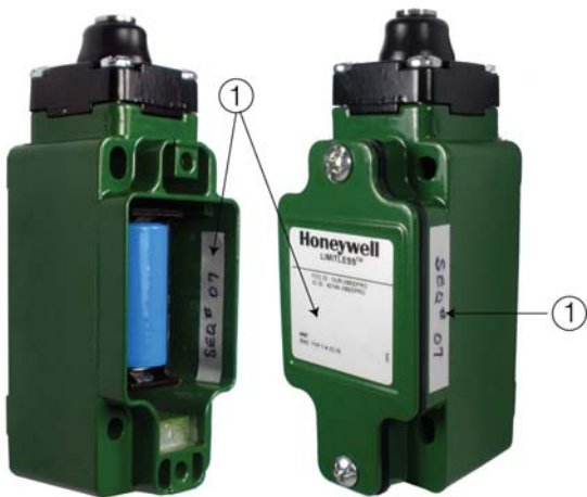
Figure 6. Limitless™ Switch Label Placement
